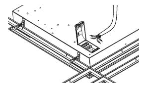
Wire the mains cable to the terminal block. Replace the reflectors. Installation complete.
