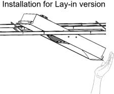
Install fitting up into ceiling grid, then wire mains into terminal block. Installation complete
